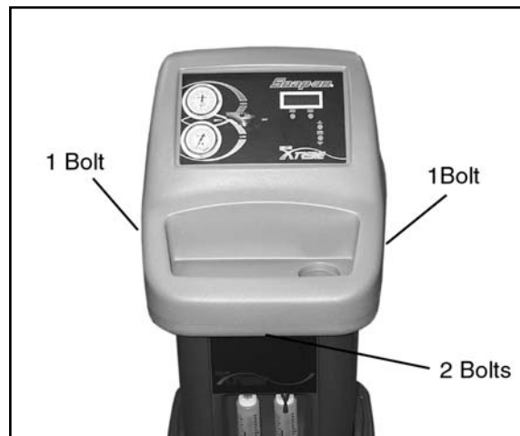
Figure 3-2: Top Cover Bolt Locations
