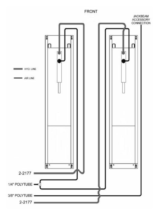
Figure 6 - Air Safety, Auxiliary Air and Hydraulic Connections
