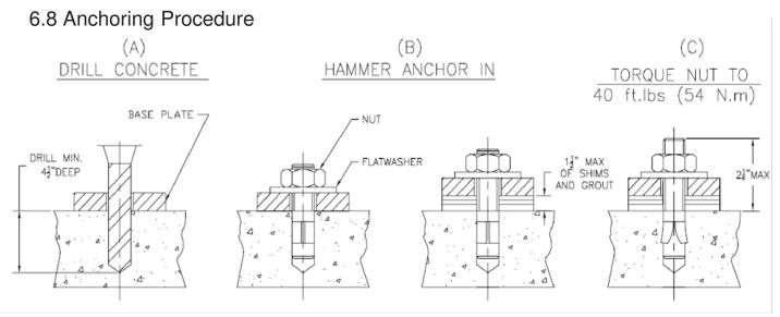
Figure 8 - Anchoring
