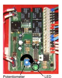
6. Repeat these steps 5-6 times to completely bleed the system of air. Check the lift for hydraulic leaks at all connections. When complete, turn the potentiometer adjustment fully counter clockwise.
