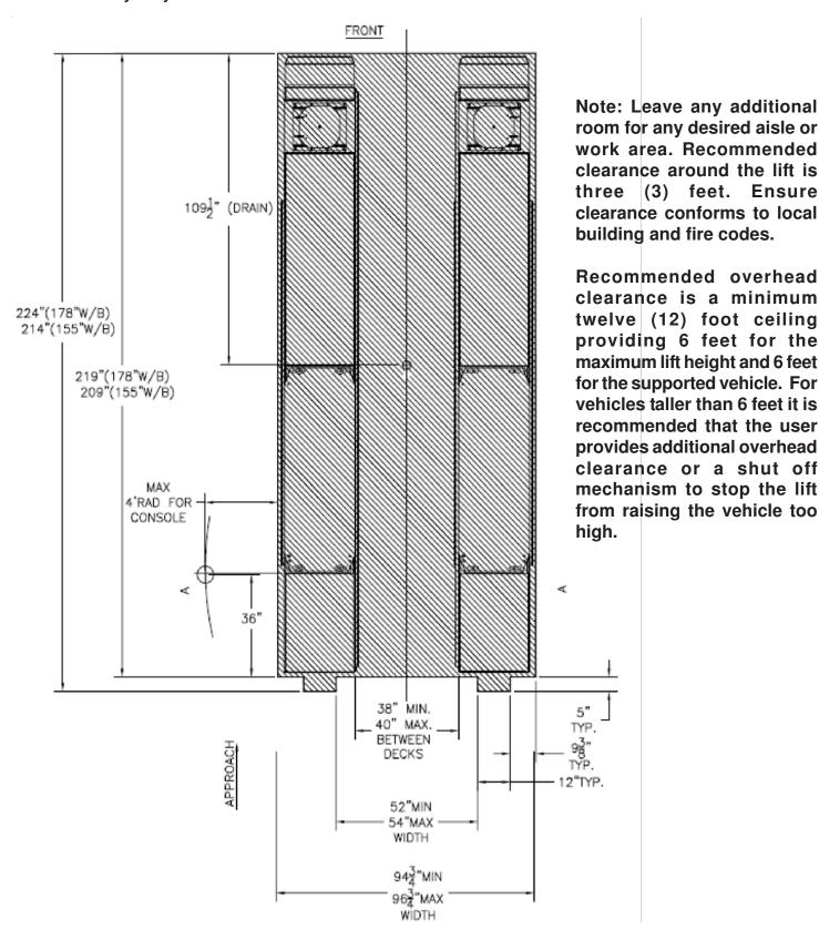
Figure 2 - Typical Bay Layout (Flush Mount)
