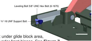
Use shims provided to support under glide block area, kicker area of baseframe and under front hinges. See Figure 7.
