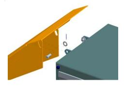
3. Install Jackbeams with reference to the Jackbeam user manual.
