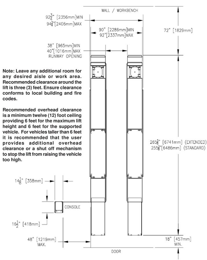
Figure 3 - Typical Bay Layout (Surface Mount)
