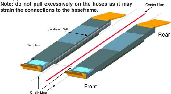
Ensure that the turnplate pockets are at the front, and that Jack Beam rails for each runway face each other.
