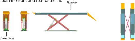
\*Check that the diagonal measurements between opposite corners of the baseframes are equal. Lower and raise the lift and repeat these measurements.
