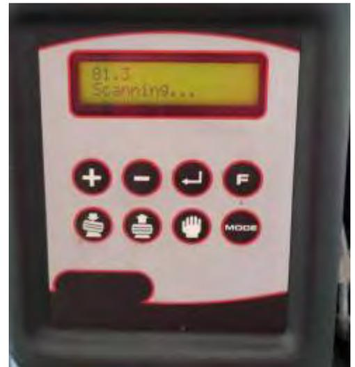
At the end of the surface scanning the procedure will save the data into internal memory and will exit from C81.
