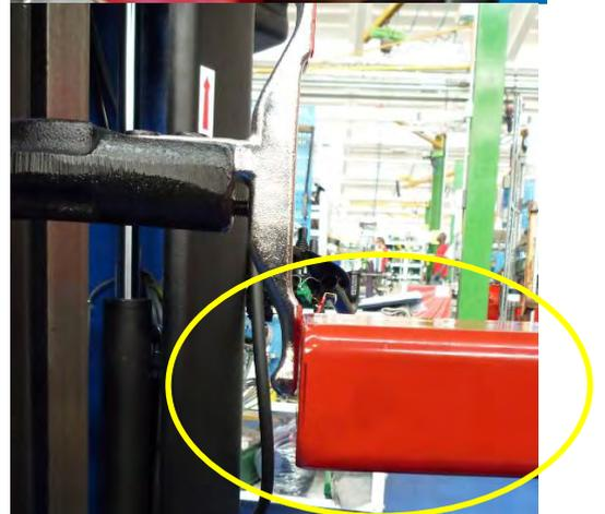
Use the horizontal motion joystick to move the calibration tool and touch gently the Tool2 plastic protection.
