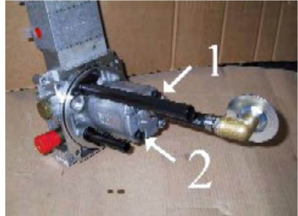
**IMPORTANT! BEFORE REPLACING THE PUMP VERIFY IF THE O RINGS #1 , #2 AND THE SEAL #3 ARE FINE.**
