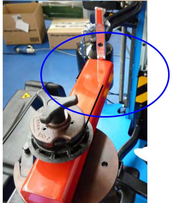
Use the vertical toolbar joystick to place the Tool2 to the Vertical centerline of the calibration tool visible in the picture below:
