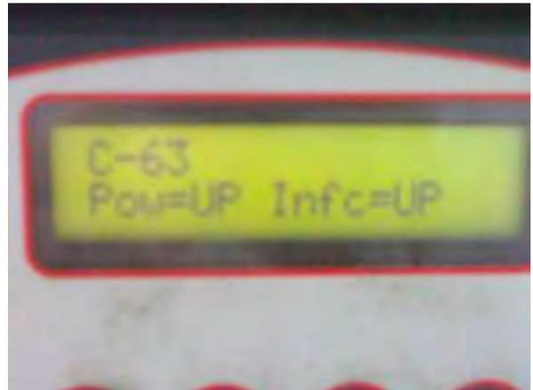
When the communication is bad from the Solenoid valve board A3 the display shows the following messages:
