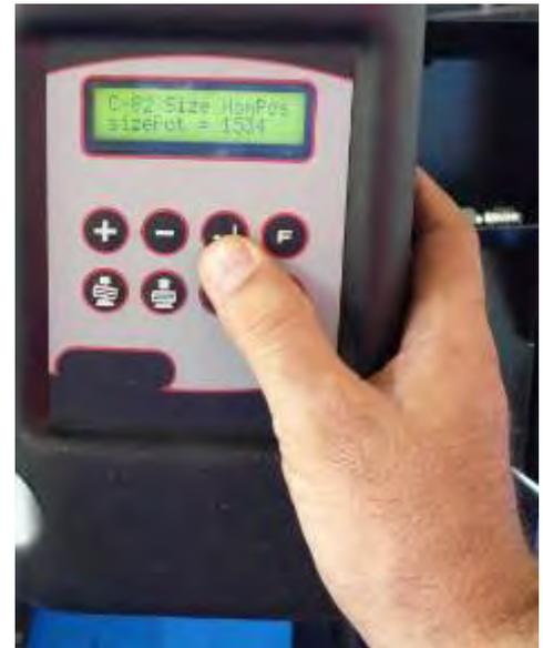
Press Enter button to store the calibration data in permanent memory and exit from C82.
