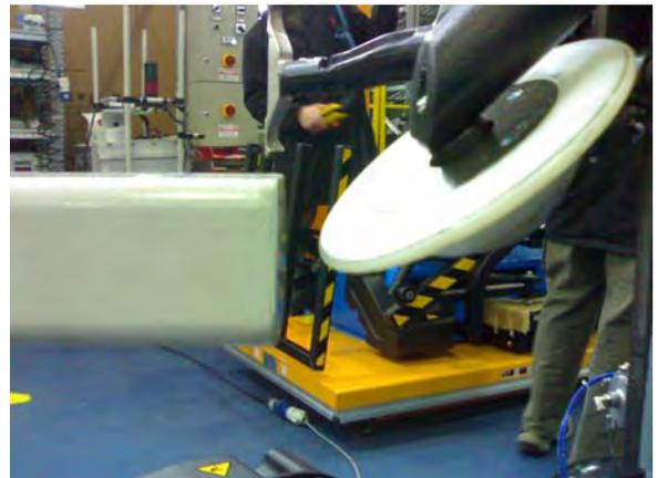
Use a tire lever and lift up the bead breaker arm up to end of stroke.
