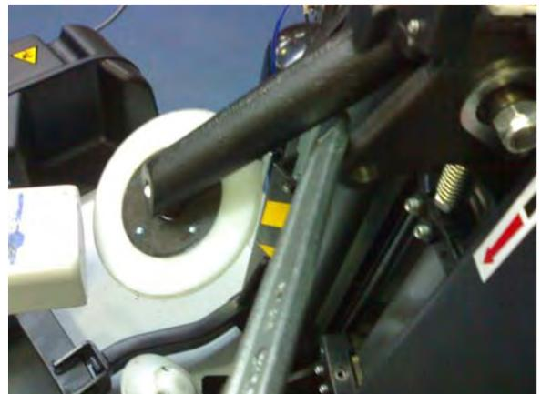
Move the centre post to get the calibration tool front plate in contact with the disk.
