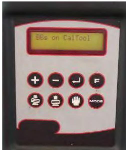
The automatic procedure moves the Bead Breaker arms to a height that is for the upper BB immediately over the calibration tool, and the lower BB immediately below the calibration tool.
