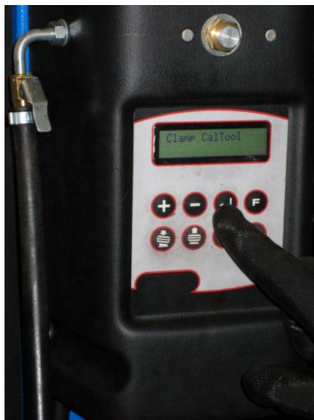
Make sure that the centering cone has clamped properly the calibration tool.
