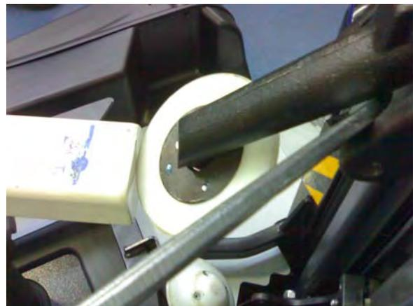
**Step 3: Front plate Calibration tool on Lower bead breaker disk.**
