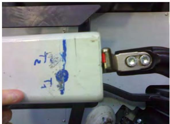
Use the vertical toolbar joystick to place the Tool2 to the Vertical centerline of the calibration tool and use the horizontal motion joystick to move the calibration tool and touch gently the Tool2 plastic protection.
