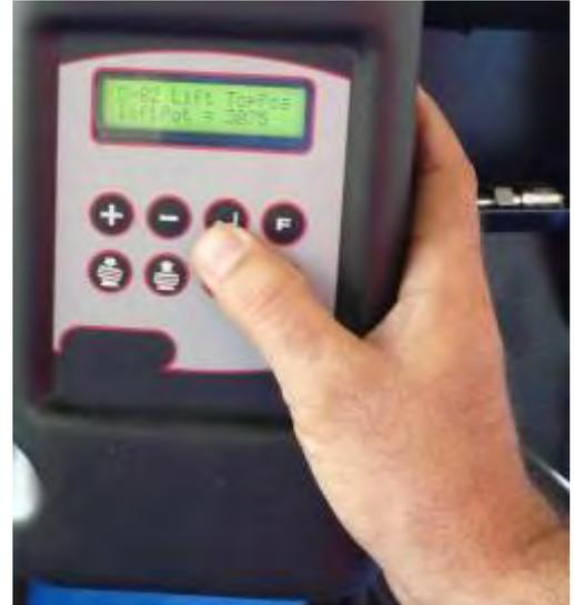
Press Enter button when in position and both lift and rotation devices go automatically to home position.
