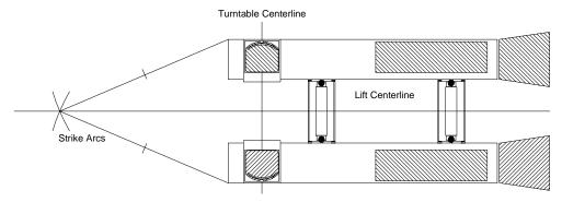
FIGURE 1. DETERMINE CENTERLINES
