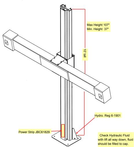
If lift won't come down: Clean velocity fuse locate @ bottom of tower. Also check pulley and cables
