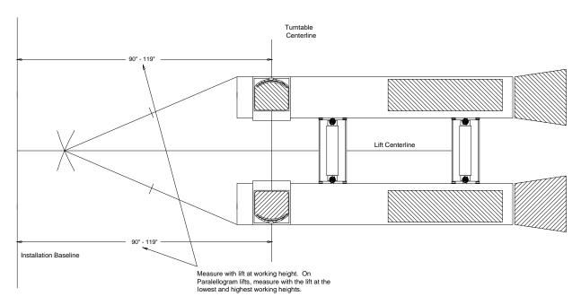
FIGURE 2. DETERMINE INSTALLATION BASELINE
